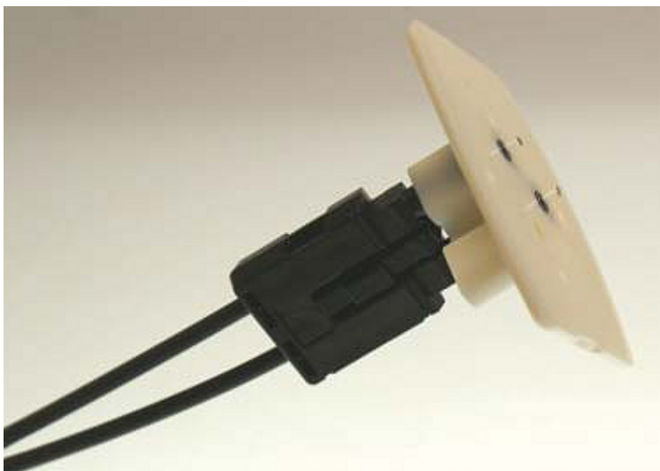
Fig. 38: Sanding gauge with protruding fiber ends
