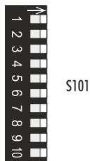
Fig. 8: DIP switch S101, switches 1 to 10.
