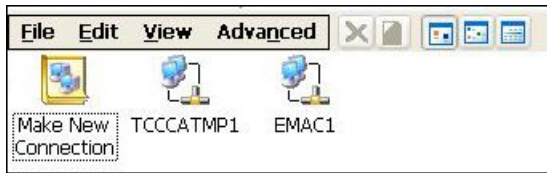
Fig. 9: Ethernet interfaces with Windows Embedded Compact 7.
