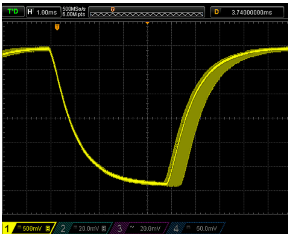
Fig. 28: EL4078 with 100 µs EtherCAT cycle time, output jitter > 1 ms
