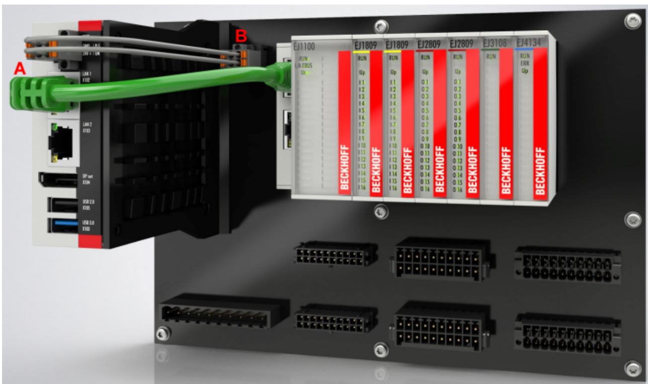
Fig. 29: Example for the connection of a C6015 IPC to an EJ system
