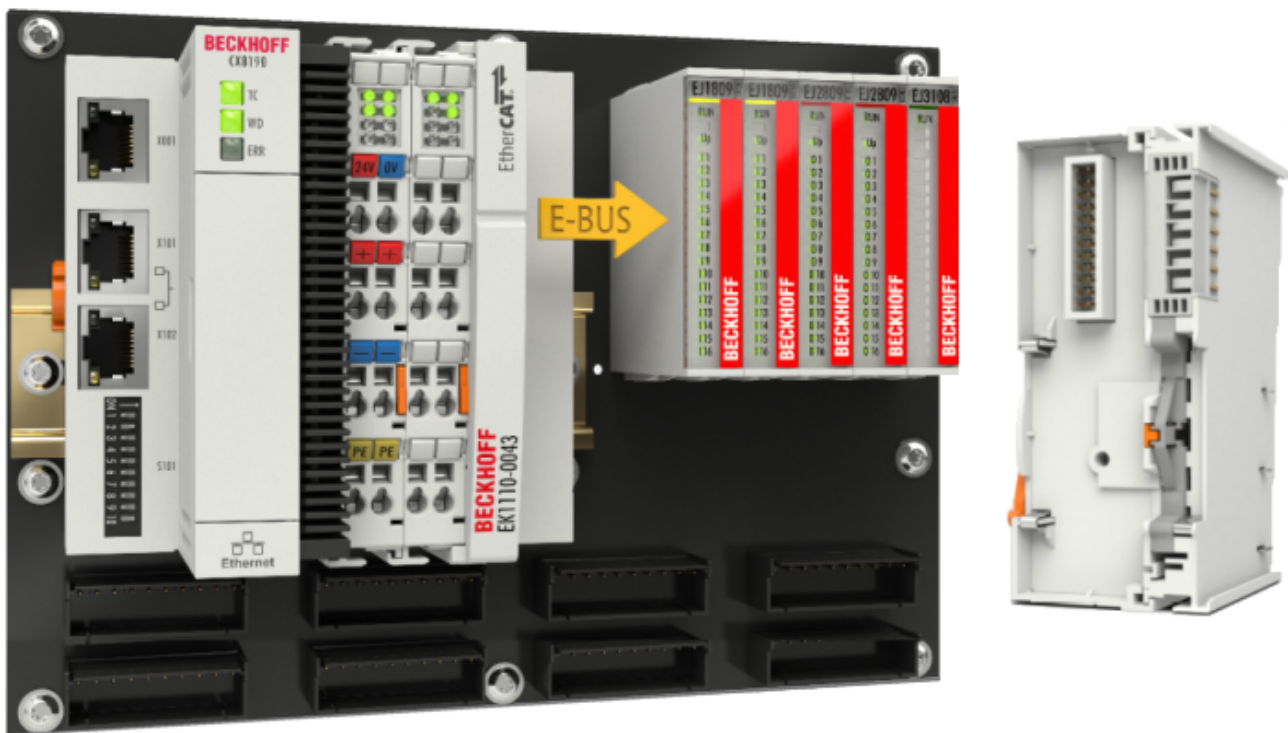
Fig. 14: PCB with Embedded PC, EK1110-0043 and EJxxxx, rear view EK1110-0043
