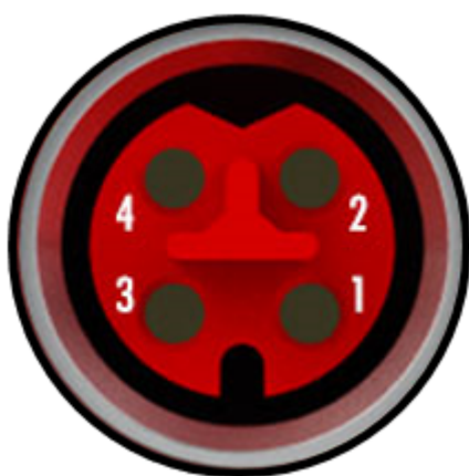
Fig. 25: Pin assignment M8, EtherCAT P In and EtherCAT P Out
