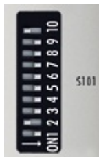
Fig. 15: DIP switch S001: left off "0", right on "1"
