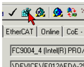
Fig. 210: Activation of the configuration
