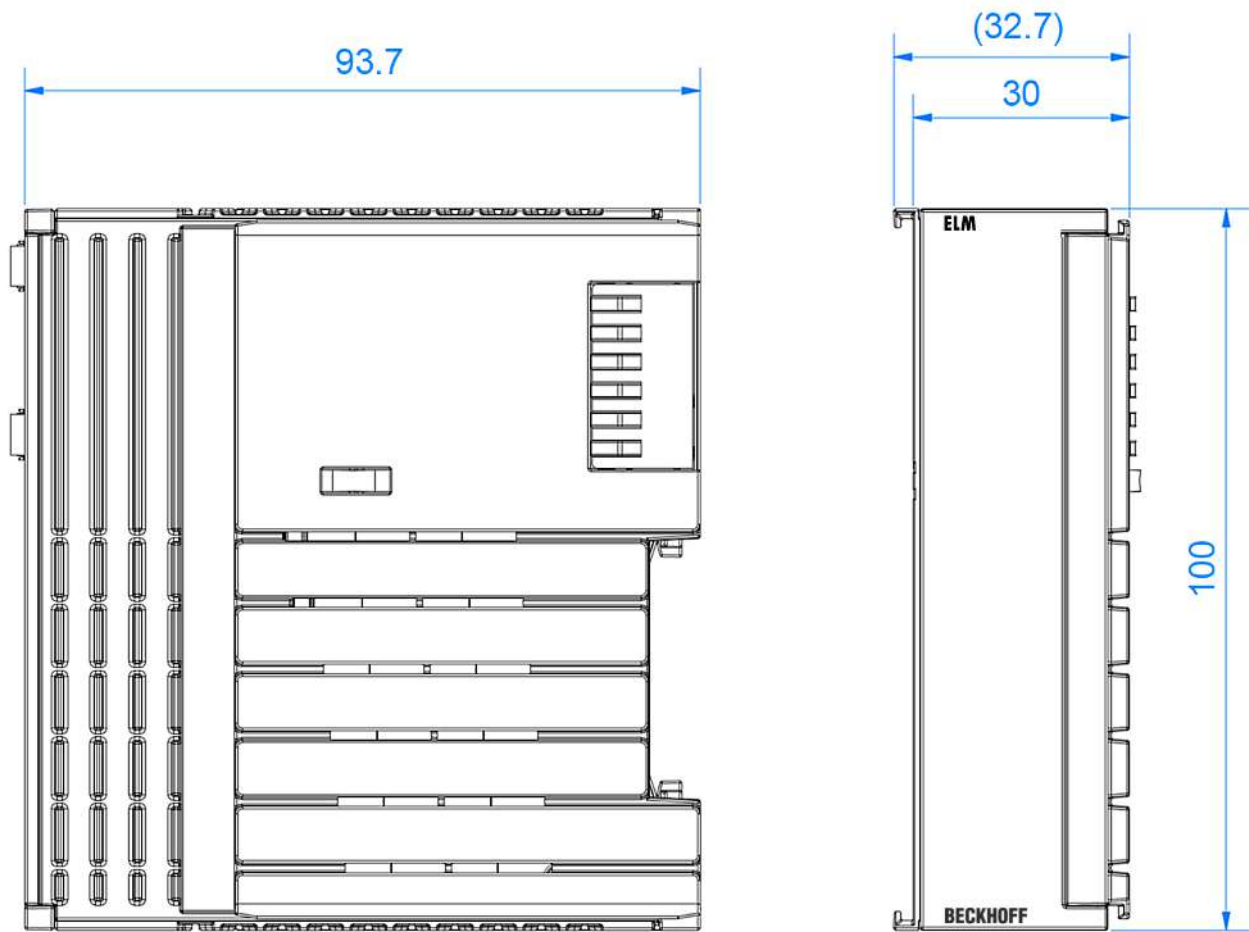
Fig. 131: Dimensions: ELM2xxx terminals
