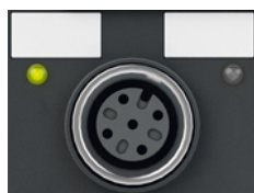
Fig. 27: Status LED on an M12 socket for EP1008-0022
