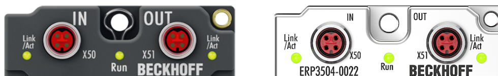
Fig. 169: Status LEDs for ethercat
