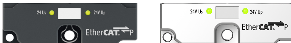
Fig. 168: Status LEDs for the power supply
