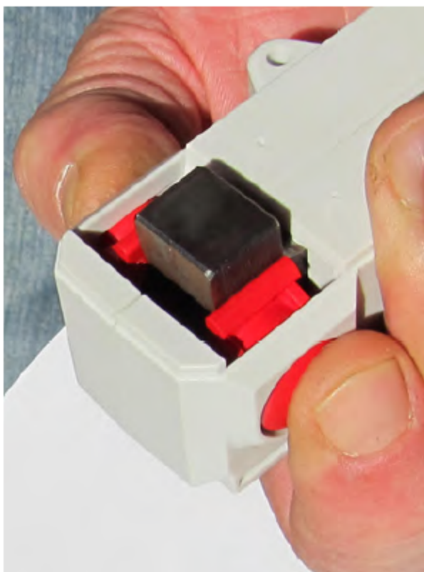
Fig. 26: Buttons to open the SCT7xxx
